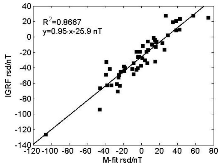
**Figure 4:** The IGRF residuals versus the normal field residuals at 53 sites. The IGRF field values have been calculated at 157 m above the sea level at 2004.5 epoch.
