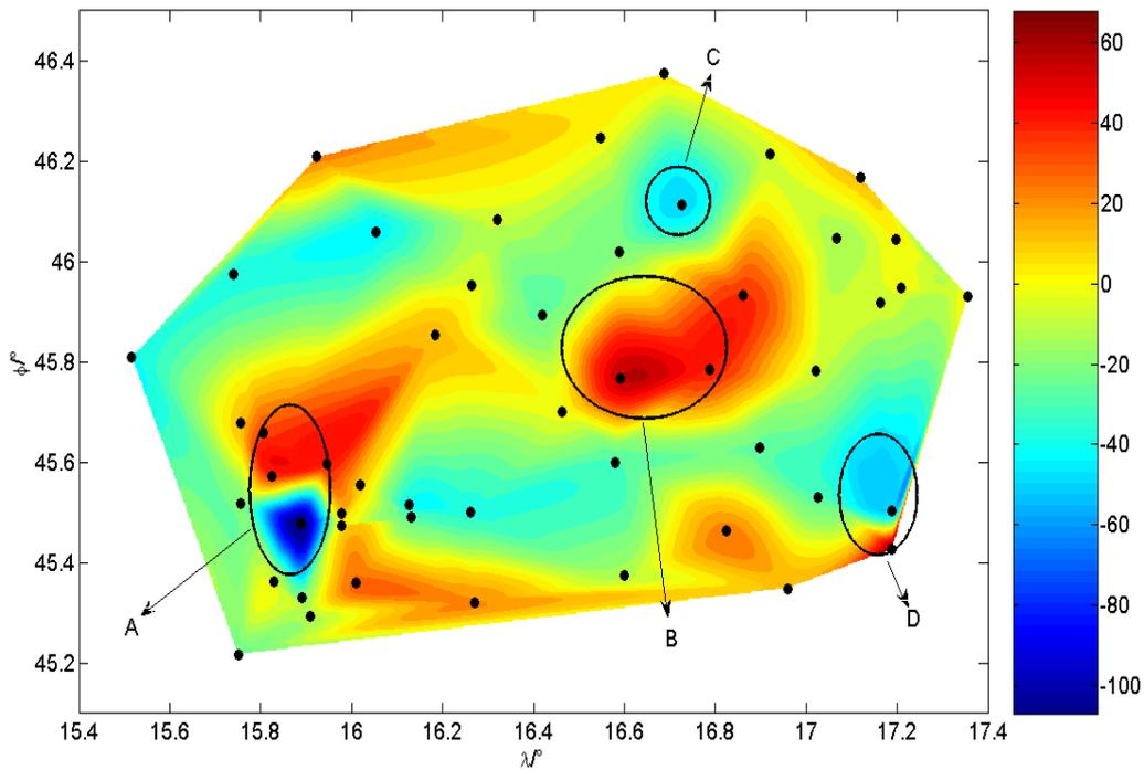
**Figure 3:** The residuals of the normal total field. The bar scale unit is nT. Survey sites are denoted with filled circles and letters A-D denote the major anomalies of residuals. Geographic latitude and longitude are denoted with  $\Phi$  and  $\lambda$ , respectively.
