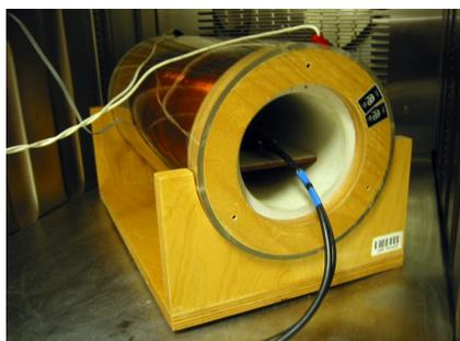
**Figure 2:** Fluxgate sensor placed in the coil.
