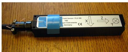
**Figure 3:** FL3-100 fluxgate sensor with a temperature sensor attached.
